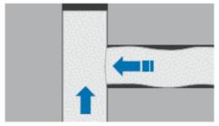
Note especially for the window assembly when cutting of the tape: the addition of at least 1 cm per meter of joint length.
