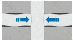
For cross and T-joints it is recommended to push the tape of the horizontal joint butt against the tape of the vertical joint. Make sure the strips do not lengthen, but abut.
